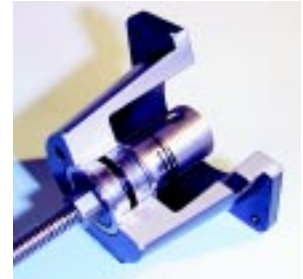
Sherline's stepper motor mounts include two preloaded bearings to eliminate end play and a damped steel coupling to protect the motor. Stepper motors are powerful 130+ oz-in, NEMA 23 frame size units.
