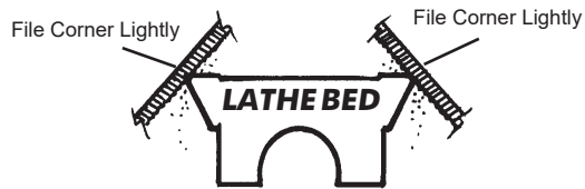
FIGURE 1—Filing corners of bed dovetail for better fit of tailstock riser block.
