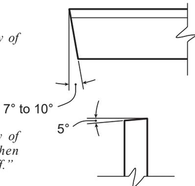
FIGURE 4—Top view of blade (enlarged) when ground for “parting off.”
