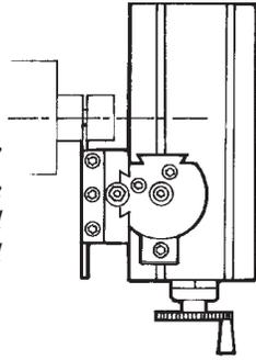
The turning speed for parting should be approximately one-half the normal turning speed for any given material. One word of caution; never use a parting tool on a part mounted between centers. The part may bind on the cutter and result in a scrapped part or a broken cutting tool.
