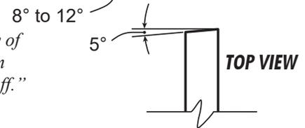
If you are sharpening the blade to “part off”, the blade should have an additional angle of approximately 5° when viewed from the top with the point on the right. (See Figure 2.) Normally the angle would be as high as 15° but the .040” thickness of the blade would not be rigid enough and the blade could bend. If you want to cut grooves, don’t put any angle on the blade when seen from the top.
