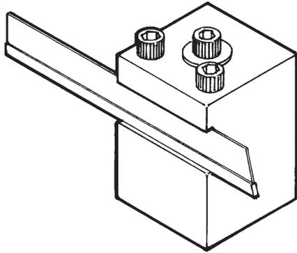
**NOTE: Always use plenty of cutting fluid when using the Cutoff Tool.**
