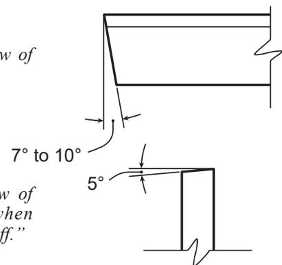
FIGURE 2—Top view of blade (enlarged) when ground for "parting off."
