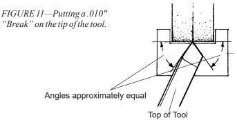
This means that if you set the tool flat on the tool rest the tool rest angle would have to be increased to get an even flat. This wouldn't be worth the effort, so the easy way is to free hand it. You should start by touching the heel of the tool first, and then change the angle until a slight flat is put on the tip. Of course, the angle you're holding it at has to be close when starting to get desired results.
