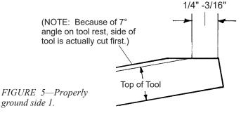
Move the blank back and forth across the face of the wheel until you have ground a  $10^{\circ}$  angle on approximately 3/16" (4 mm) of side 1.
