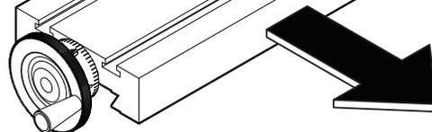
FIGURE 1—Mount the extended T-nuts (P/N 40250) in the T-slot closest to the headstock.
