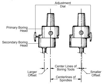
FIGURE 2—Reversing the lower portion of boring head for large or small holes.
