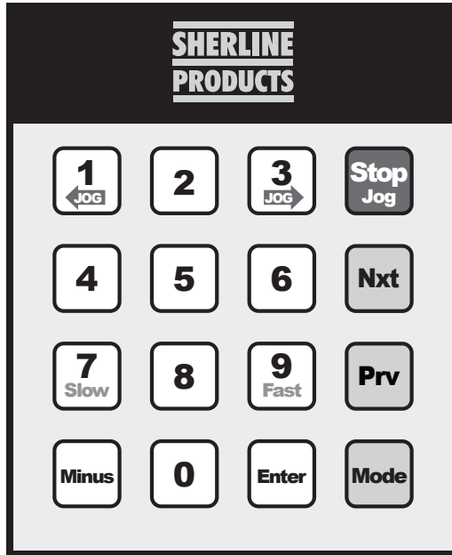
FIGURE 4—Layout of the keypad.
