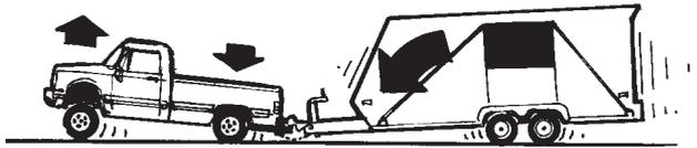
*Top heavy loads can cause trailer "dive" under hard braking, possibly reducing control.*
