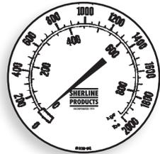
*The gauge reads in both pounds on the outer ring and the equivalent reading in kilograms on the inner ring.*
