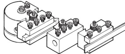
**P/N 2250 Quick-Change Tool Post and Holder Set**—A dovetailed steel tool post accepts steel holders for a 1/4"
