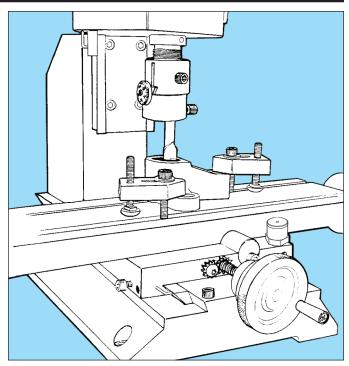
FIGURE 5— Boring the inside of a hole to exact size with a boring tool held in a boring head.
