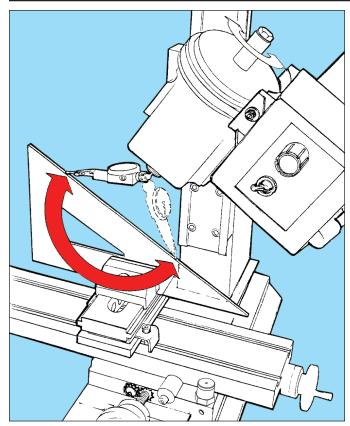
FIGURE 9—Indicating in a  $30^{\circ}$  head tilt using a mill vise and draftsman's triangle
