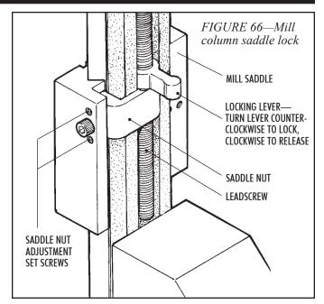
present between the handwheel and the leadscrew thrust. To eliminate this, push down on the saddle to make sure the handwheel is fully seated against the thrust. Double check your height adjustment. Now, when milling, the saddle cannot move any further down.
