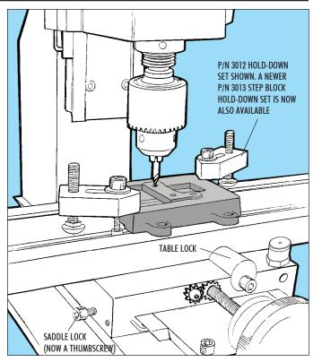
FIGURE 2—Large or odd shaped parts are usually clamped to the mill table as shown here. Smaller parts can be held in a milling vise. Here a center drill is used to accurately locate the holes to be drilled in a clamped part.
