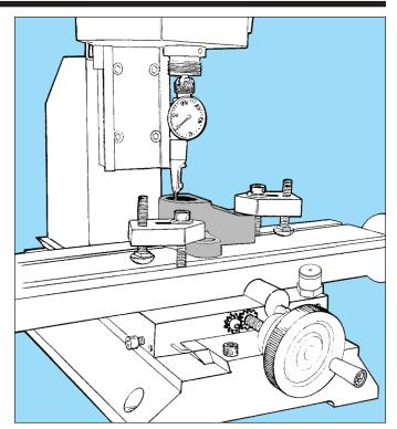
FIGURE 7—Indicating in the center of a hole.
