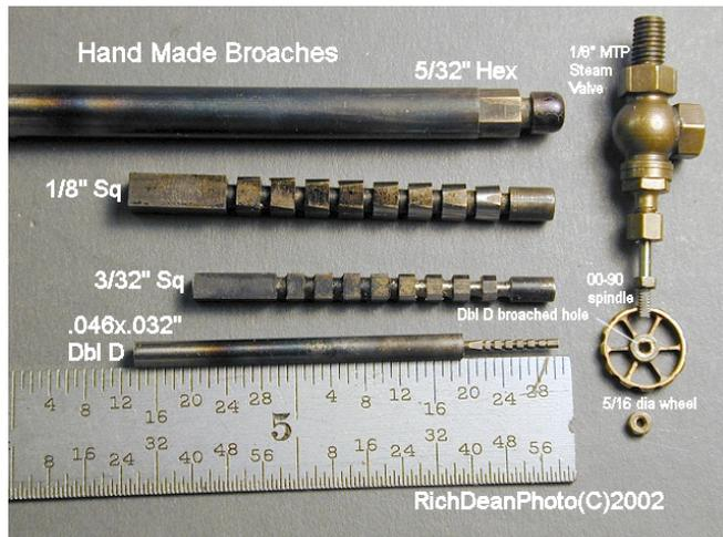
The broaches shown above are plain lathe turned, propane torch hardened and tempered in oil. You will have to decide the overall size, shank and dimensions to use for your particular project. Use W1, O1 or whatever drill rod (tool steel). No reason to be fussy.
