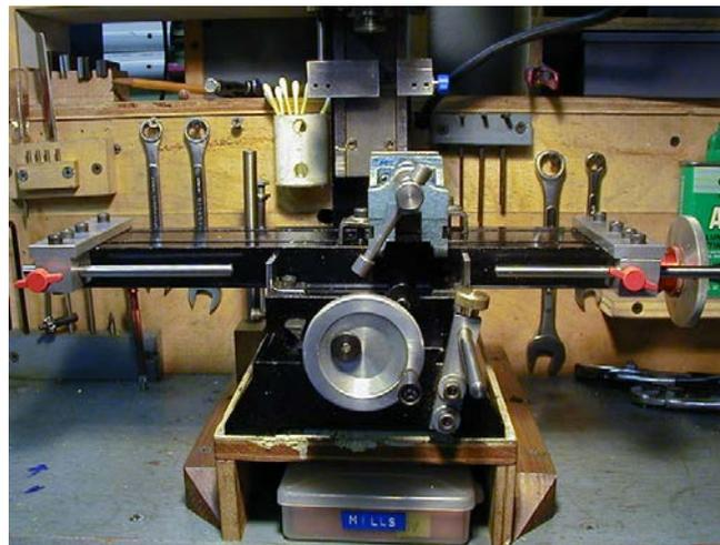
*The left-hand photo shows the Y-axis depth stop. Here Tracy tried a knurled brass knob to lock the bar but felt it couldn't be tightened enough to keep the rod from moving. He now uses screws with a larger plastic handle for more leverage but suggests a small piece of brass between the end of the screw and the rod will protect the surface of the rod. In the right-hand photo both the Y-axis and X-axis locks can be seen.*
