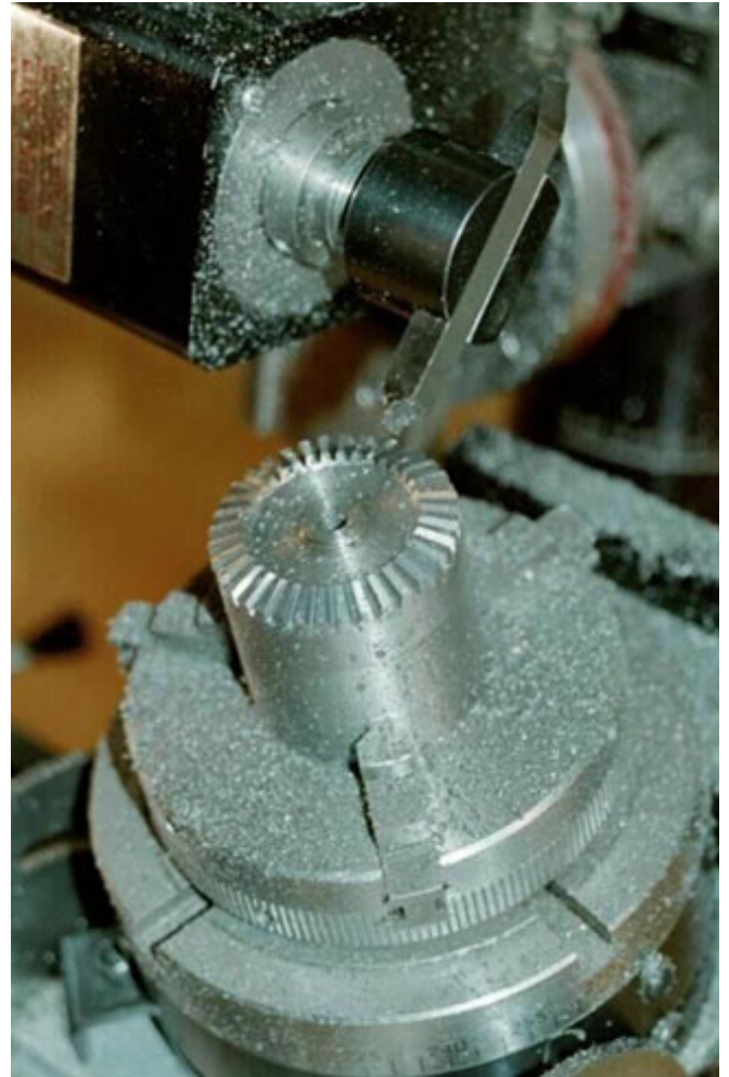
Here is the gear after I parted it off and am relieving the back of the gear to remove unnecessary metal. You need to be very careful with how deep you cut on the back so you don't cut all the way through (this is more of that steep learning curve I mentioned earlier ;-).
