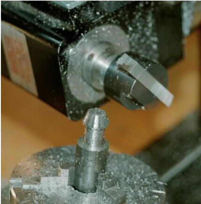
Here is the finished pinion back on the lathe with the shaft turned down.
