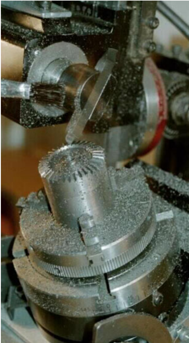
Here is the gear on the final pass.
