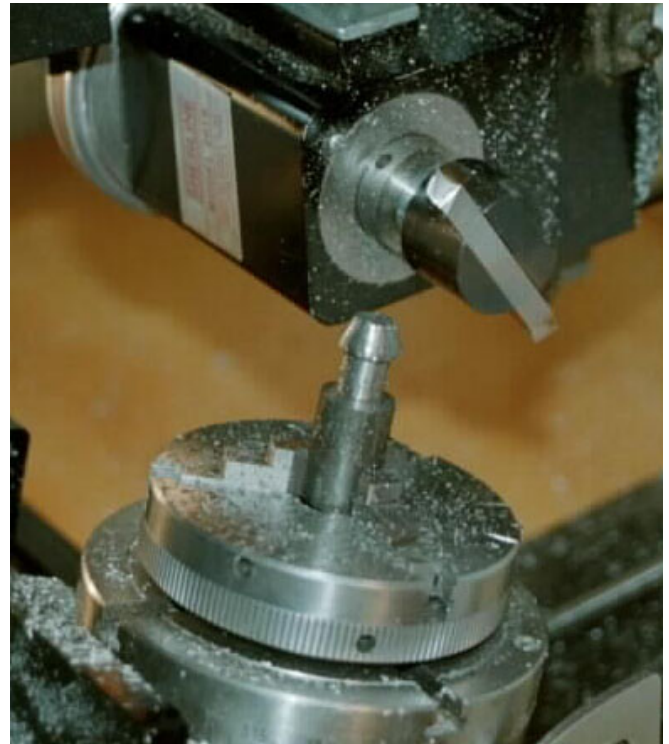
Here is the pinion after the first round of cuts.
