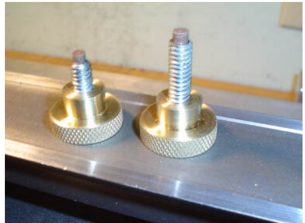
FIGURE 5—shows the two Delrin tipped, knurled screws
