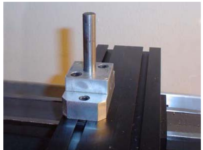
The above photos show Jim's adjustable toolpost grinder. It holds a Dremel tool and can position the grinder at any angle. (Click on any photo for larger image.) The photos should give you enough info to build your own. Jim didn't make any drawings.
