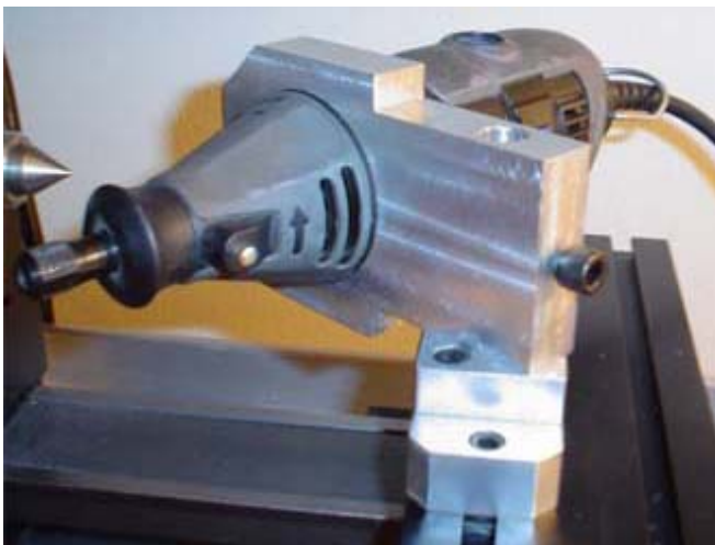
The above photos show Jim's adjustable toolpost grinder. It holds a Dremel tool and can position the grinder at any angle. (Click on any photo for larger image.) The photos should give you enough info to build your own. Jim didn't make any drawings.
