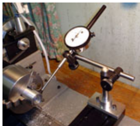
(L) An indicator stand is turned on the lathe using a 4-jaw chuck. (R) The stand mounts to the crossslide table using standard T-nuts.
