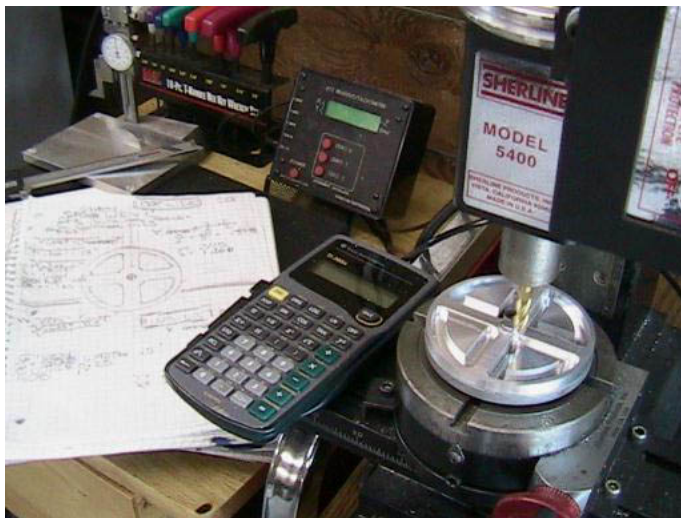
Photo 4 — The wheel blank is held to the rotary table using a 10-32 screw and washer in the center hole that has been drilled into the chuck adapter.
