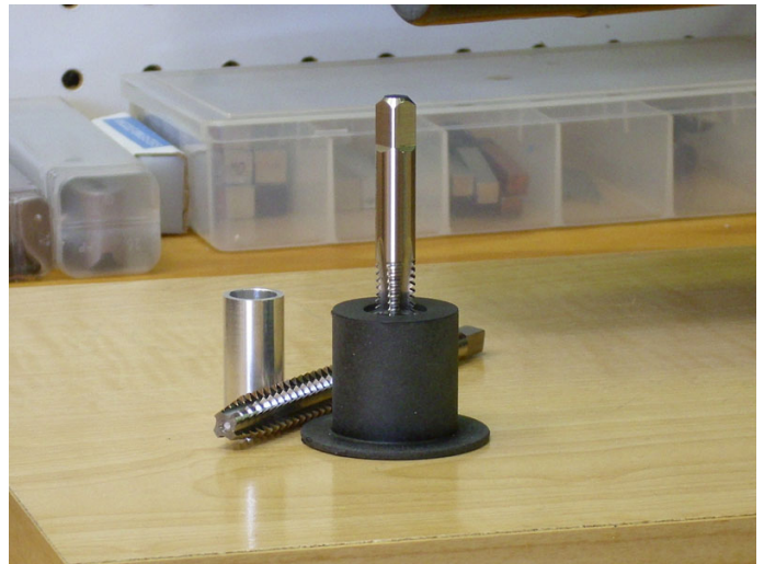
Photo 3—The guide block is seen with one of the inserts in place and one of another size next to its tap. The center hole is made .001" larger than the tap for a precise slip fit.
