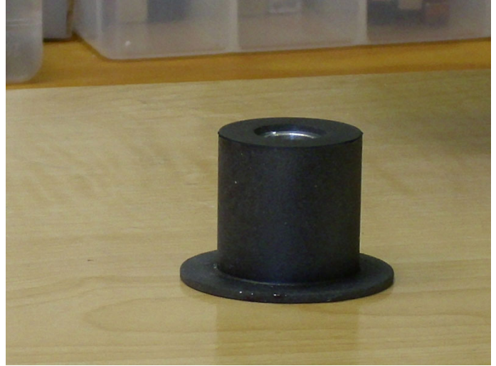
Photo 2—The plastic body with one of the aluminum tap guide inserts in place.
