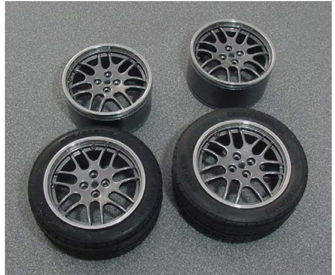
*Mark is now working on a seventh model of the Lotus 7. It will include more detail and custom made metal parts than any car he has made in the past. In honor of the seventh seven, notice the custom seven-spoke aluminum wheels he has machined. They include valve stems with separate cores that move within the stem just like the real thing.*
