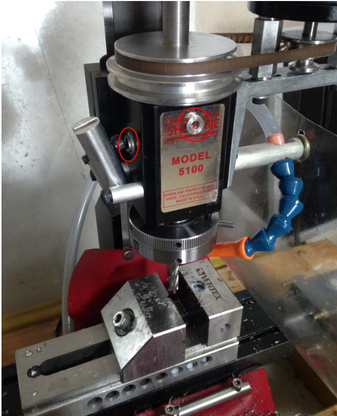
Figure 3—mill setup, open position (magnets circled in red)
