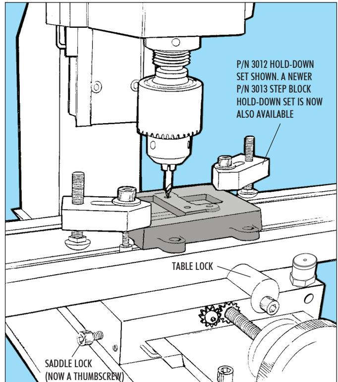
FIGURE 2—Large or odd shaped parts are usually clamped to the mill table as shown here. Smaller parts can be held in a milling vise. Here a center drill is used to accurately locate the holes to be drilled in a clamped part.
