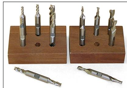
FIGURE 11— 4- and 2-flute double-ended end mill sets.
