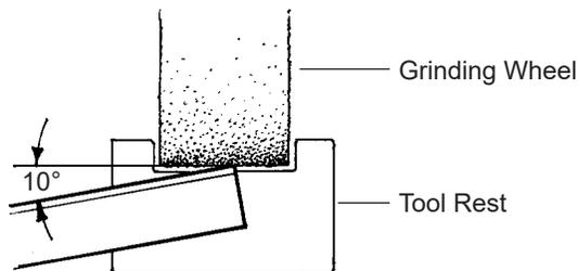
FIGURE 4—Grinding Side 1.
