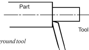
FIGURE 7—Properly ground tool cutting into a corner
