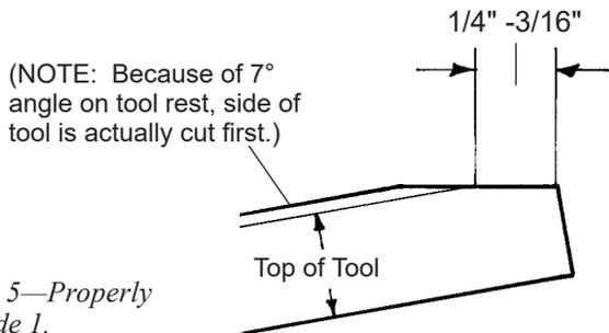
FIGURE 5—Properly ground side 1.
