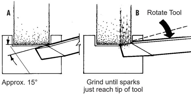
FIGURE 9—Grinding the “Hook” into side 3. When grinding tools by hand, on average, the cutting-tip surface of the tool is going to be .005” to .0010” below the top of the tool. This will leave a .010” to .020” tit on the end of your tool when facing off the part.
