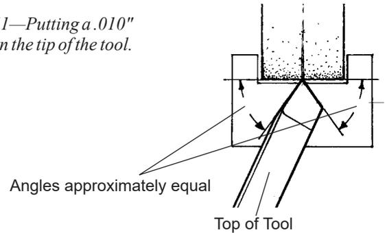
This means that if you set the tool flat on the tool rest the tool rest angle would have to be increased to get an even flat. This wouldn’t be worth the effort, so the easy way is to free hand it. You should start by touching the heel of the tool first, and then change the angle until a slight flat is put on the tip. Of course, the angle you’re holding it at has to be close when starting to get desired results.
