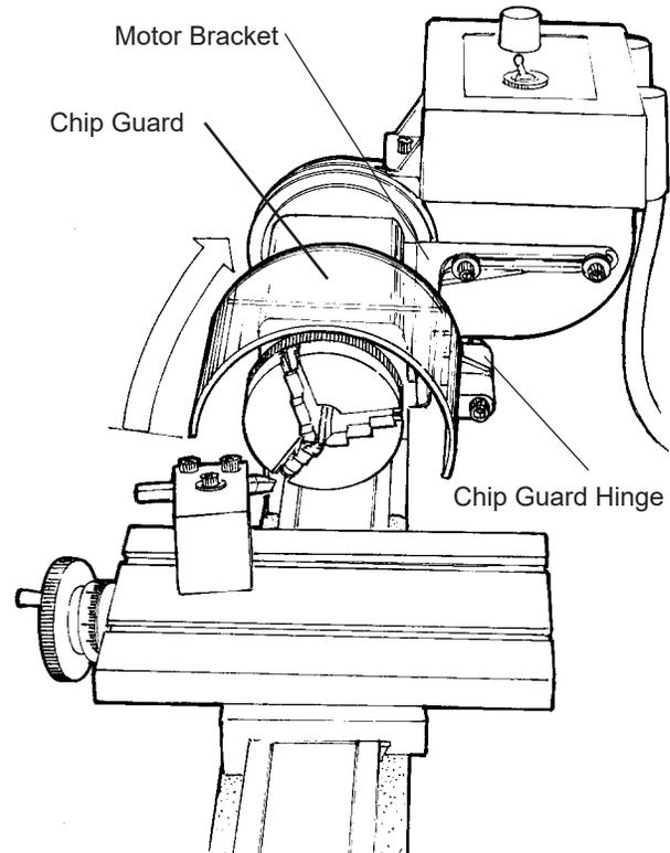
FIGURE 1—The chip guard mounted on a Sherline lathe. The guard pivots up out of the way for access to the spindle area.
