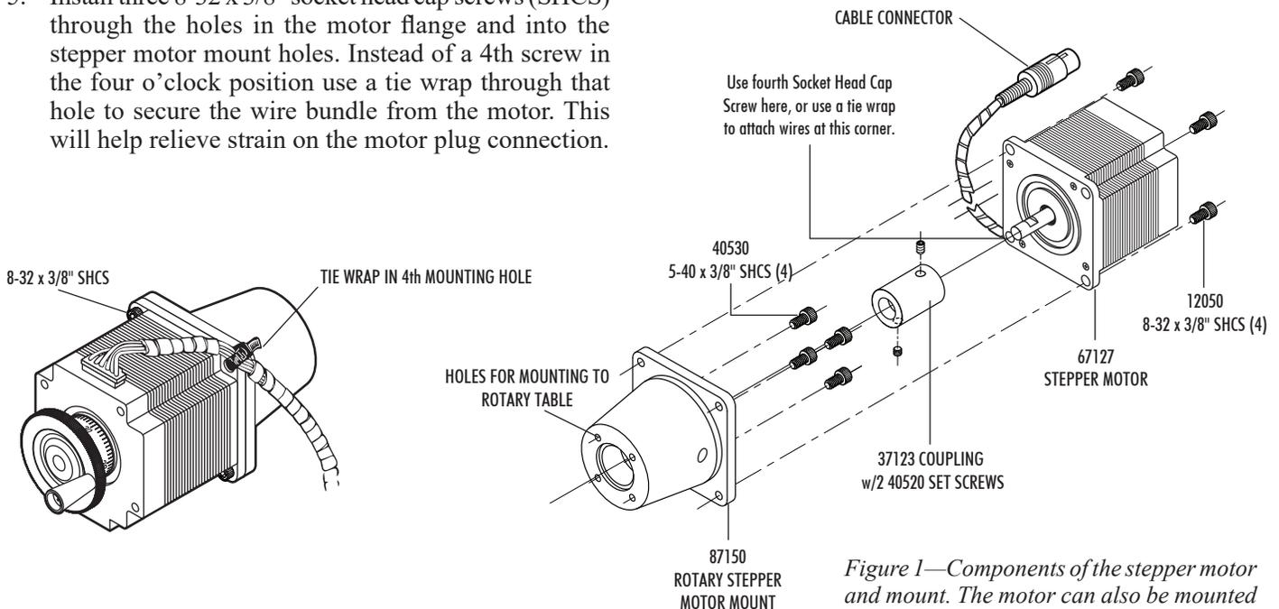
Figure 1—Components of the stepper motor and mount. The motor can also be mounted with the electronic cable facing downward.
