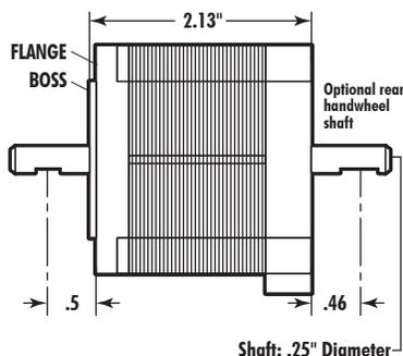
FIGURE 1—Locations for the flats on the stepper motor shaft.
