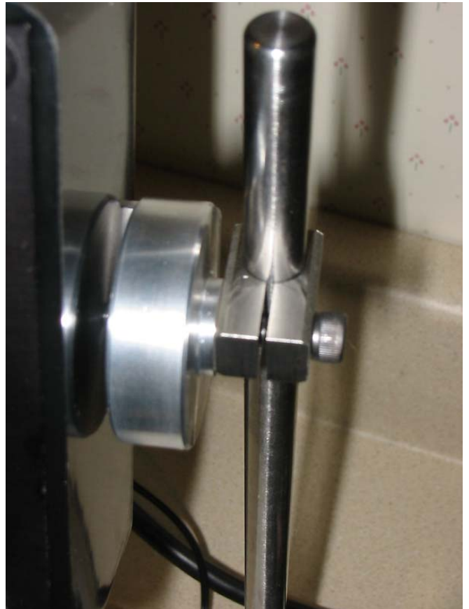
Photo 6: A top view of the adjustment system shows the slit in the piece that slides on the shaft. The vertical shaft is 12" long because Ron has a 15" tall Z-axis on his mill in place of the standard 11" column. For normal height mills the rod could be shorter than 12".
