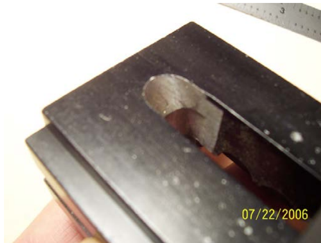
Photo 2—Seen from the top of the vise, a chamfered area allows the hold-down screw to extend farther back.
