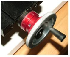
An inch handwheel (left) has 50 marks, each indicating .001" of actual table travel. A metric handwheel (right) has 100 marks. When used on an inch machine, each of the 100 marks now indicates .001" removed from the diameter of the part. Shown are adjustable zero handwheels.
