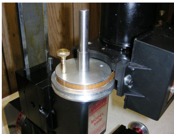
Jerry's spindle lock and rod for tapping stamp held in 4-jaw chuck
