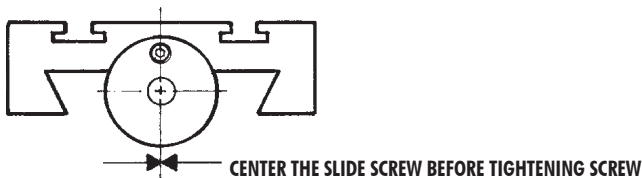
FIGURE 2—Making sure the crossslide screw is centered
