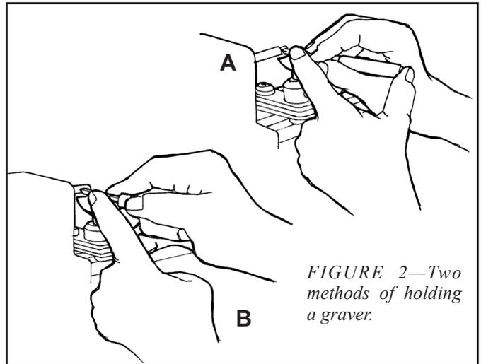
FIGURE 2—Two methods of holding a graver.
