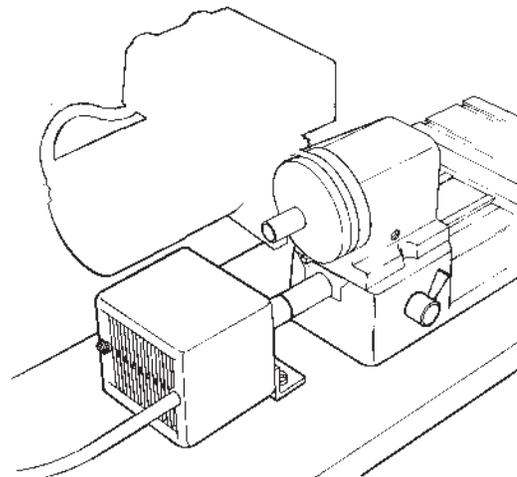
FIGURE 2—Power feed installed on base.
