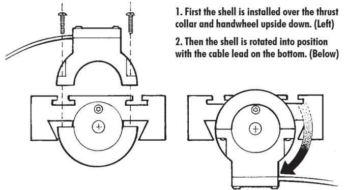
1. First the shell is installed over the thrust collar and handwheel upside down. (Left)
