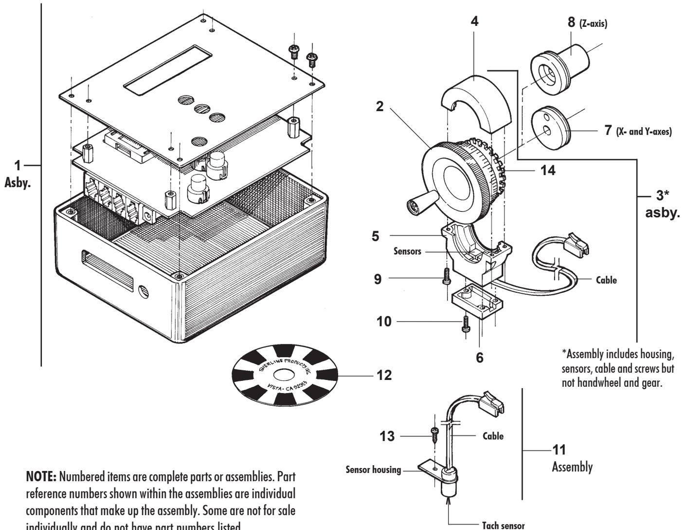
**NOTE:** Numbered items are complete parts or assemblies. Part reference numbers shown within the assemblies are individual components that make up the assembly. Some are not for sale individually and do not have part numbers listed.
