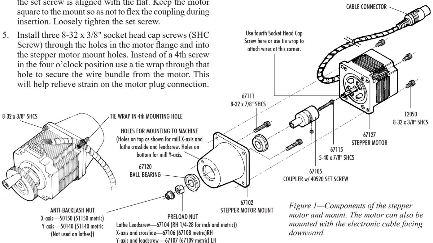
Figure 1—Components of the stepper motor and mount. The motor can also be mounted with the electronic cable facing downward.
