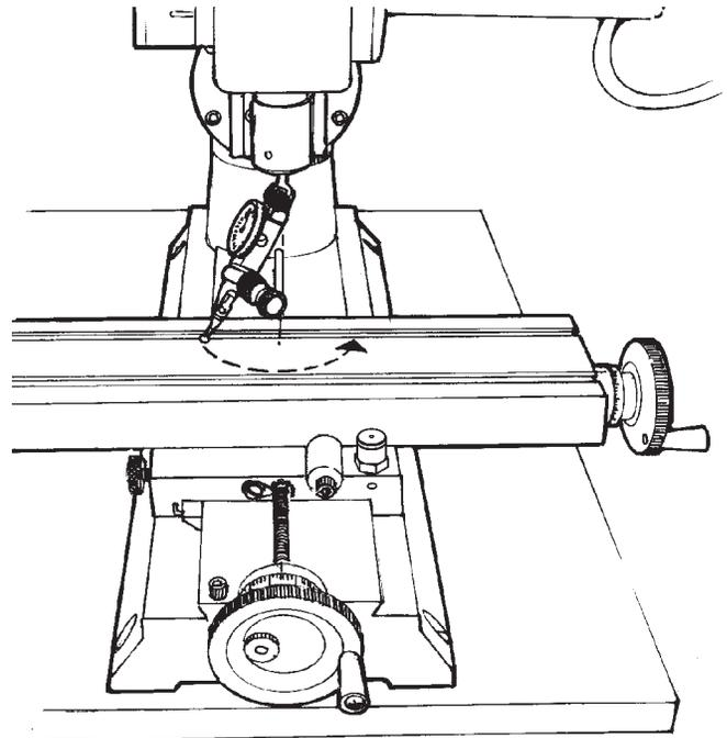
FIGURE 4—Squaring the left to right rotation of the column with the X-axis
