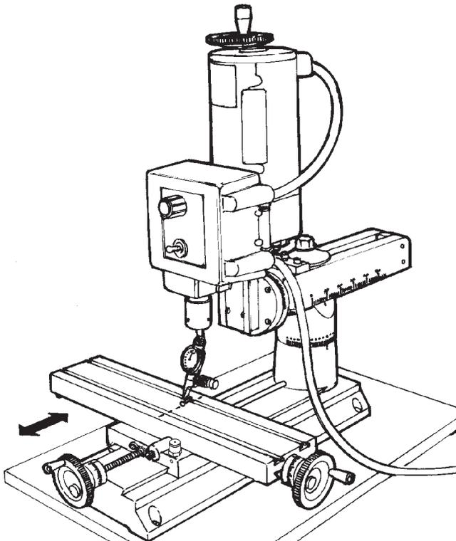
FIGURE 2—Checking for built in error in the table travel along the Y-axis
