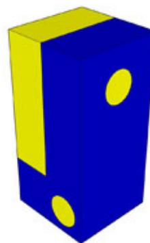
The finished lock is clamped to the front flange on the Sherline lathe saddle using a set screw. The lower brass nut locks the saddle against the bed to secure the Z axis. The upper brass nut locks against the side of the table to lock the X axis. The lock can be left in place, as it does not interfere with other operations when not needed. To make it easier to visualize the part, Vince did these CAD drawings. Blue represents the part while yellow shows the metal to be removed.
