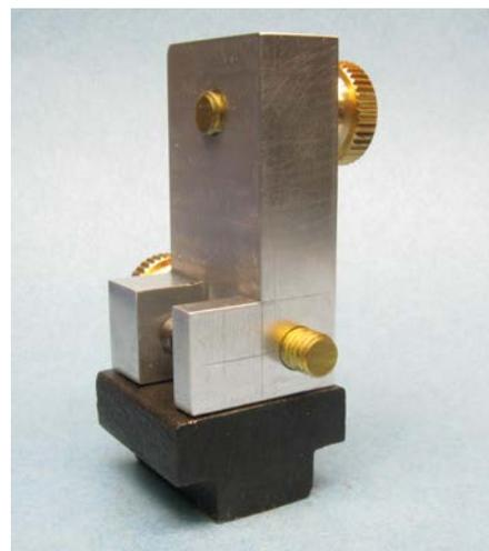
The first drawing shows the dimensions, while the other two show the finished parts. The knurled brass knobs on the attachment screws are a professional touch. They are bonded to the threaded brass rod using Loctite permanent liquid adhesive. The knobs are available for use on electrical contact posts if you don't want to make your own. Brass is used to keep from damaging the surfaces of the bed and table.
