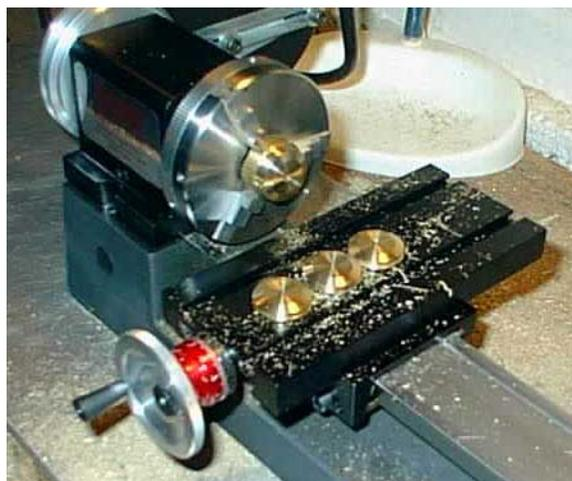
*These two photos show Keith's setup to turn the taper and O-ring grooves on the train's wheels.*
