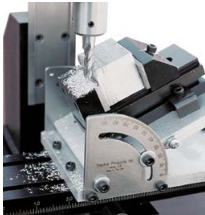
Chamfers can be milled using the tilting angle table on a mill.
