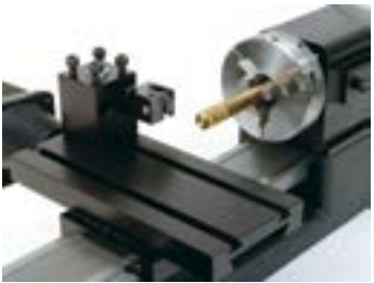
The bump knurling tool holder mounted on the CNC crossslide.
