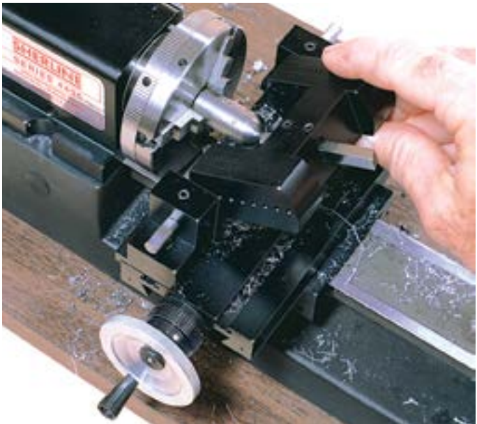
The radius cutting attachment can cut a convex or concave radius. Unlike most lathe operations, the tool is moved up and down rather than horizontally.
