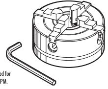
NOTE: P/N 1030, 1032 and 1044 chucks are independent jaw chucks. Each jaw is adjusted individually. 4-jaw self-centering chucks are available in both 2.5" and 3.1" sizes. See P/N 1075, 1076 and 1078. P/Ns 1032 and 1078 chucks have a 22 x 1.5 mm thread for use on ER-16 collet spindles.
