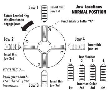
difficult part of replacing the jaws is engaging the scroll thread and first tooth of each jaw without binding. Never use force when replacing the jaws, and if binding occurs, simply back up the scroll slightly and wiggle the jaw until it is free to move in the slot. Advance the scroll counterclockwise and engage jaw #3 next in the slot that previously held jaw #1 (the slot marked "A"). Continue to engage jaws 2 and finally jaw 1.
