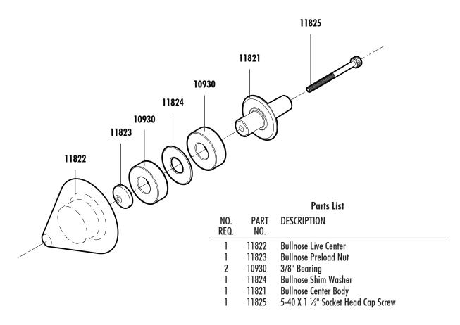
NOTE: The bearings are pressed in at the factory. Preload on the bearings is adjusted before the nose piece is installed. Once assembled, the 1182 Bullnose Live Center is not considered user-serviceable. Parts are shown for reference only.
