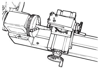
FIGURE 1—Cutting a simple taper with the compound slide eliminates the need to rotate the headstock.
