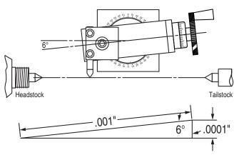
FIGURE 5—Compound rest set for precision cross-feed adjustment.
