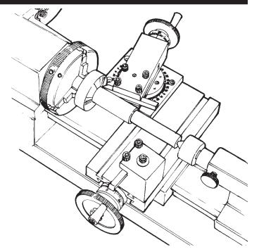
FIGURE 2—The compound can also be offset to allow cuts to be taken close to the chuck. It would be more difficult to hold this piece between centers and cut the taper by offsetting the headstock as might normally be done. Take light cuts when the compound overhangs the table like this.
