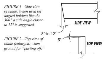
If you are sharpening the blade to "part off", the blade should have an additional angle of approximately 5° when viewed from the top with the point on the right. (See Figure 2.) Normally the angle would be as high as 15° but the .040" thickness of the blade would not be rigid enough and the blade could bend. If you want to cut grooves, don't put any angle on the blade when seen from the top.
