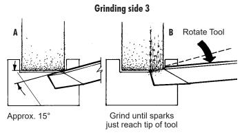
FIGURE 9—Grinding the "Hook" into side 3. When grinding tools by hand, on average, the cutting-tip surface of the tool is going to be .005" to .0010" below the top of the tool. This will leave a .010" to .020" tit on the end of your tool when facing off the part.
