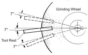
FIGURE 2—Set tool rest at any height, but at 7° angle from centerline of wheel.
