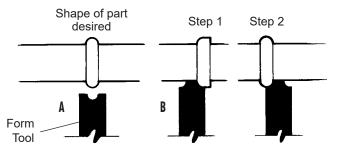
FIGURES 14A—A typical form tool made by a custom tool making shop, and 14B, a home shop method of achieving the same finished shape in two steps with a tool that can be ground on a bench grinder.
