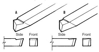
FIGURES 10A—Normally recommended "hook" ground into tool and 10B, Simpler method suggested for Sherline tools.
