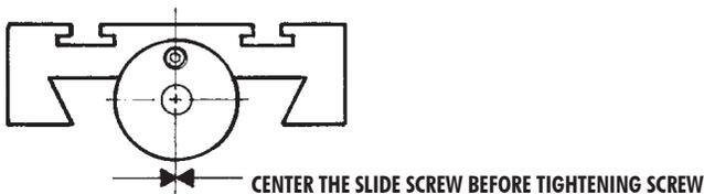
FIGURE 2—Making sure the crossslide screw is centered
