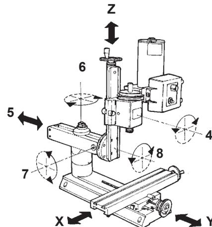
**FIGURE 1**—Directions of movement of a multi-direction column. Although a Model 2000 mill is shown here, the same movements are achieved on the lathe by using the crossslide handwheel as the X-axis and the leadscrew handwheel as the Y-axis.
