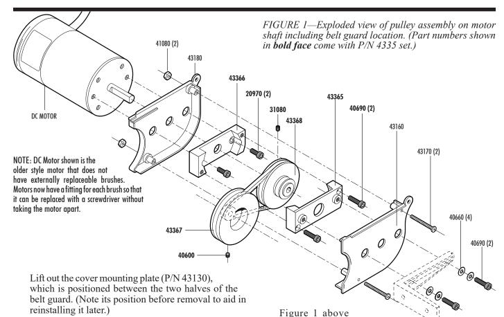
3. Remove the two long screws (P/N 43170) that go through the belt guard and take off the outer belt guard (P/N 43160). (Make sure you don't lose the nuts [P/N 41080] that are inset into the rear belt guard. They may stick in the holes or they may fall out.)
