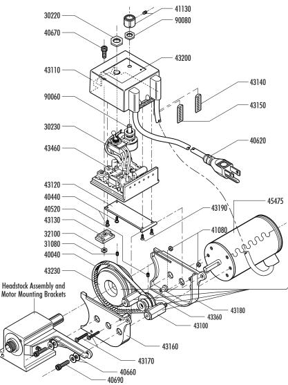
existing hole in the belt housing using the existing self-tapping screw. Drill the other end to accept a small through bolt and nut to hold the sensor. The middle "leg" of the bracket should be about 5/16" in depth. The sensor is mounted 90° to its previous position with its face as close as possible to the pulley decal without touching it.
