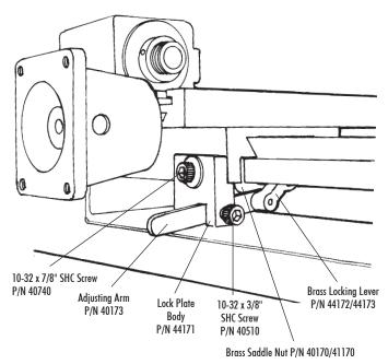
FIGURE 1—Components of the lever locking system as they are now installed on new Sherline CNC lathes.
