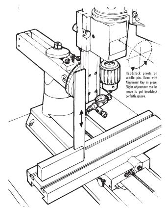
FIGURE 6—Fine tuning the headstock rotation alignment with a machinist's square and dial indicator
