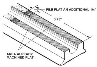
FIGURE 7—On older columns, file the top end of the mounting surface of the bed flat. You will be extending the machined flat surface an additional 1/4" or so for a total of 3-3/4" of flat.
